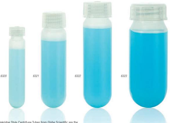
These new Oakridge Style Centrifuge Tubes from Globe Scientific are the economic choice for high speed refrigerated or non-refrigerated centrifugation. Molded from durable, chemical resistant polypropylene, the tubes have round bottoms and consistent wall thicknesses for centrifugation at up to 50,000g when filled to 80% of their nominal capacity. Oakridge style tubes are autoclavable and re-usable and are designed with leakproof linerless closures.
